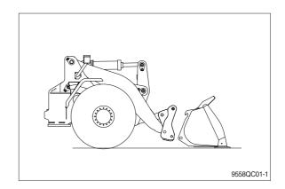
(2) Tilt quick coupler forward and align the upper attaching points of the quick coupler with upper attaching points on the bucket. Raise the boom until the bucket rests in the quick coupler and tilt the quick coupler rearward until the bucket is level.
